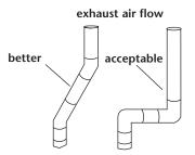
Select the route that will provide the straightest and most direct path outdoors. Plan the installation to use the fewest number of elbows and turns.
